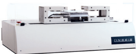
TFA with permanent magnet (up to 0.5 Tesla)
