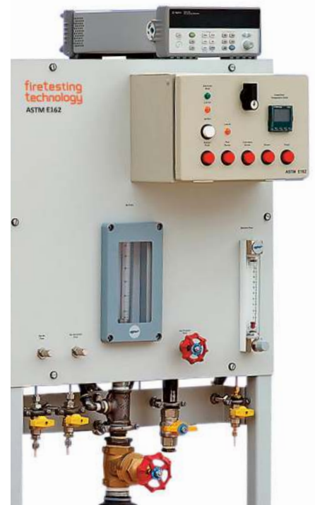
Gas Panel, Control Box and Data Logger
