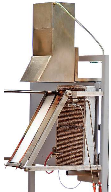
Radiant Panel, Specimen Holder and Exhaust Stack
