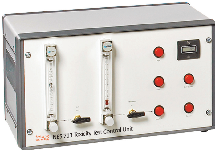
The Control Unit houses the flowmeters, timer, methane and air controls
