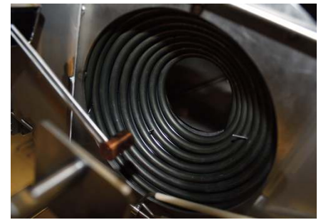
Base view of the conical heater
