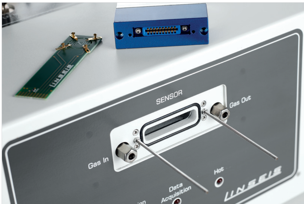
Exchangeable Sensors with an EPROM on it for easy plug and play usage.
